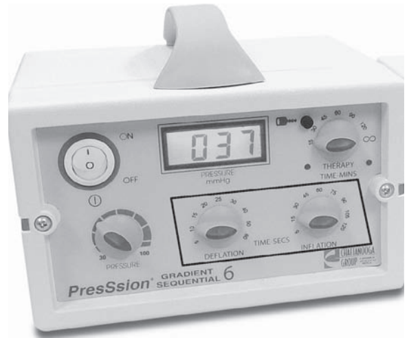
Figure 11–7 Time setting control knobs for on and off cycles of an intermittent compression unit. This illustrates the setting at the beginning of the treatment when the appliance is uninflated. The off-time knob is increased when the proper inflation pressure is reached.
