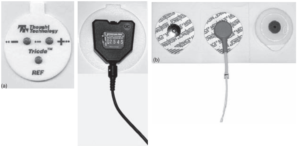
Figure 7-6 Biofeedback electrodes. (a) Both active and reference poles can be housed in a single electrode (Courtesy Thought Technology, Ltd. www.thoughttechnology.com . Copyright © 2008 Covidien AG or an affiliate. All rights reserved. Reprinted with permission.) or, (b) there can be 3 separate electrodes.
