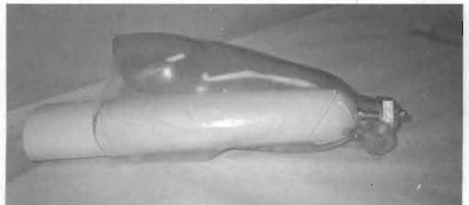
FIG. 21-2 A suspension sleeve with a pin attachment on its end can be rolled onto the residual limb, requiring less fine motor hand function.
