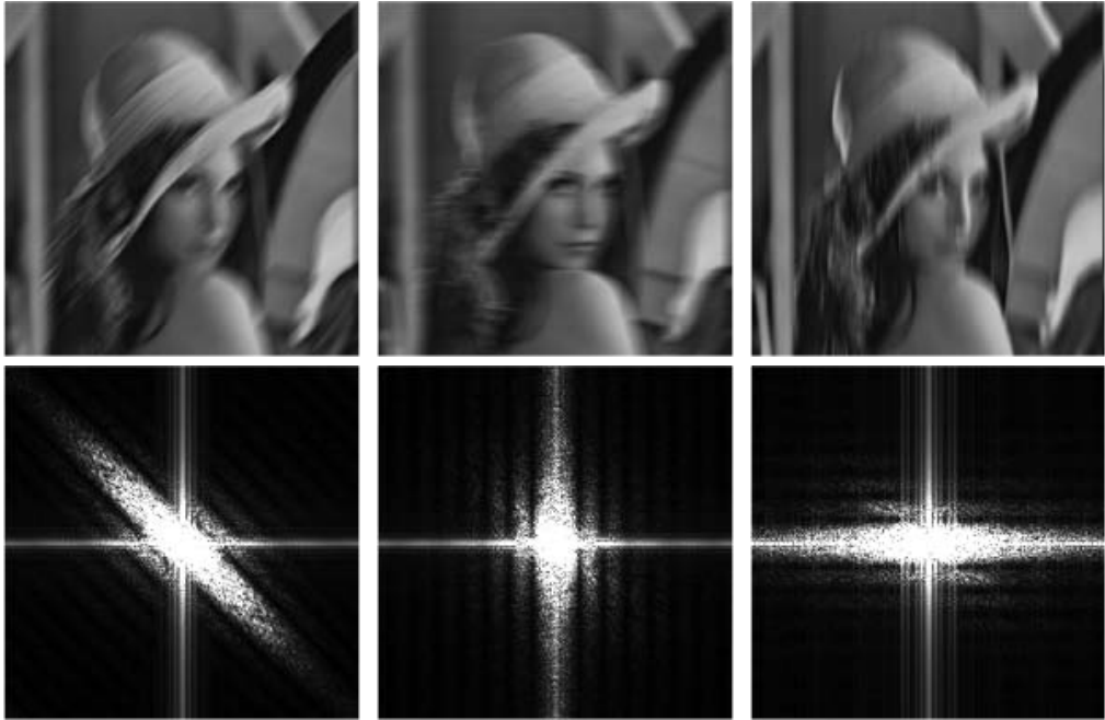
FIGURE 8.10 Frequency spectra of blurred images: (top) three differently blurred images, and (bottom) magnitude of their frequency spectra.
