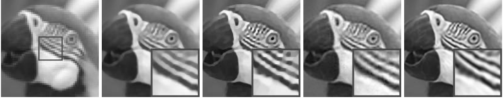
Figure 5.9 Reconstructed HR Parrots images ( \sigma_n = 0 ). From left to right: input LR image; softcut [80] (PSNR = 27.99 dB); TV [81] (PSNR = 27.85 dB); Sparsity [82] (PSNR = 28.70 dB); Algorithm 2 in [83] (PSNR = 30.46 dB)
