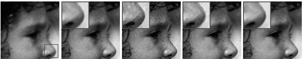
Figure 5.8 Reconstructed HR Girl images ( \sigma_n = 5 ). From left to right: input LR image; softcut [80] (PSNR = 31.30 dB); TV [81] (PSNR = 29.86 dB); Sparsity [82] (PSNR = 30.71 dB); Algorithm 2 in [83] (PSNR = 31.85 dB)
