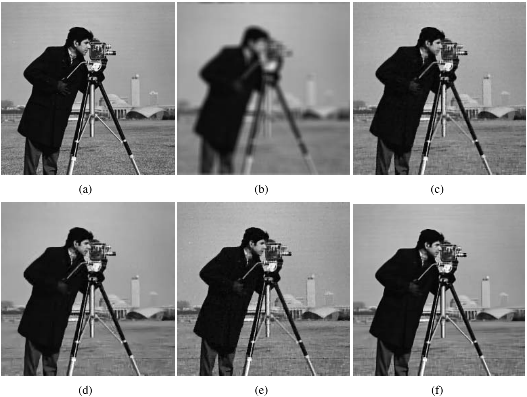
Figure 5.5 Comparison of original cameraman image, noisy blurred image ( BSNR = 40 dB, 9 \times 9 uniform blur) and deblurred images by different algorithms): (a) original; (b) noisy blurred; (c) TVMM [77] ( ISNR = 8.42 dB); (d) SADCT [78] ( ISNR = 8.57 dB); (e) TwIST [11] ( ISNR = 8.65 dB); f) CSR [79] ( ISNR = 10.60 dB).
