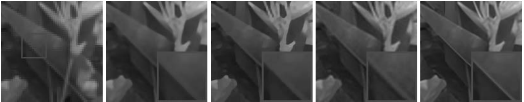
Figure 5.7 Reconstructed HR Plants images ( \sigma_n = 0 ). From left to right: input LR image; softcut [80] (PSNR = 31.19 dB); TV [81] (PSNR = 31.34 dB); Sparsity [82] (PSNR = 31.55 dB); Algorithm 2 in [83] (PSNR = 33.42 dB)
