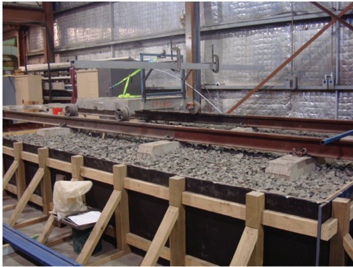
Model track used for non-destructive testing
