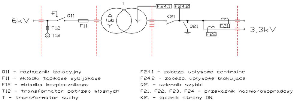
Figure 2.1. Schematic (one-wire) diagram of the transformer station type EH-d31-2600/6,0/3,3/02.01.
