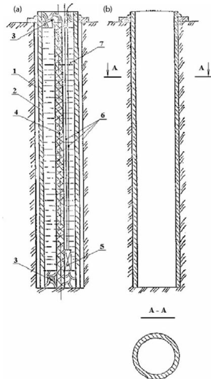
Figure 1. Structure of a shell tube (a) and tubular rock bolt TA1 (b): 1 - blasthole; 2 - shell tube; 3 - clay cap; 4 - detonating cord DCA or DCB; 5 - electrical detonator; 6 - electrical wires; 7 - filling compound (sand, water).
