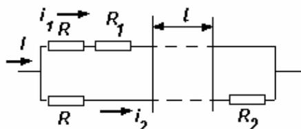
Figure 3. Circuit providing current redistribution under conductors connection.
