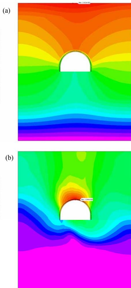
Figure 2. Distribution diagrams of displacements in system “stratified massif-support of a working” at decreased strength characteristics and increased deformation characteristics of all adjacent rock layers: (a)  $H = 200$  m; (b)  $H = 600$  m.
