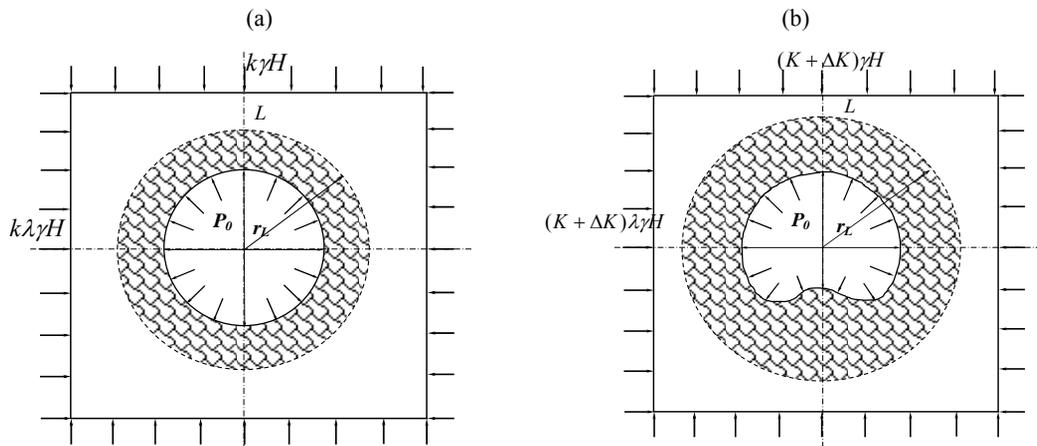
Figure 4. The solution scheme for problem of elasto-plastic stability losses: (a) an initial state of system ( $r_L < r_L^*$ ); (b) the disturbing state of system ( $r_L \geq r_L^*$ ).
