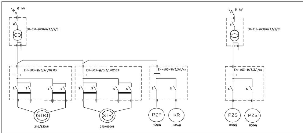
Figure 2.2 (d). The schematic diagram of the power supply system for the high-performance longwall set of equipment operated at the Lublin Coal “Bogdanka” plc.
