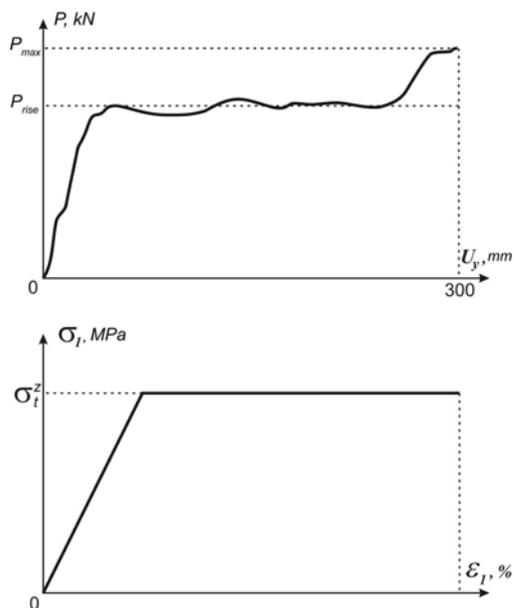
Figure 5. Substantiation of a yield lock model of a frame support made of SCP: (a) deformation-load characteristics of the real construction of a lock; (b) full diagram of deformation of the lock simulator's material.
