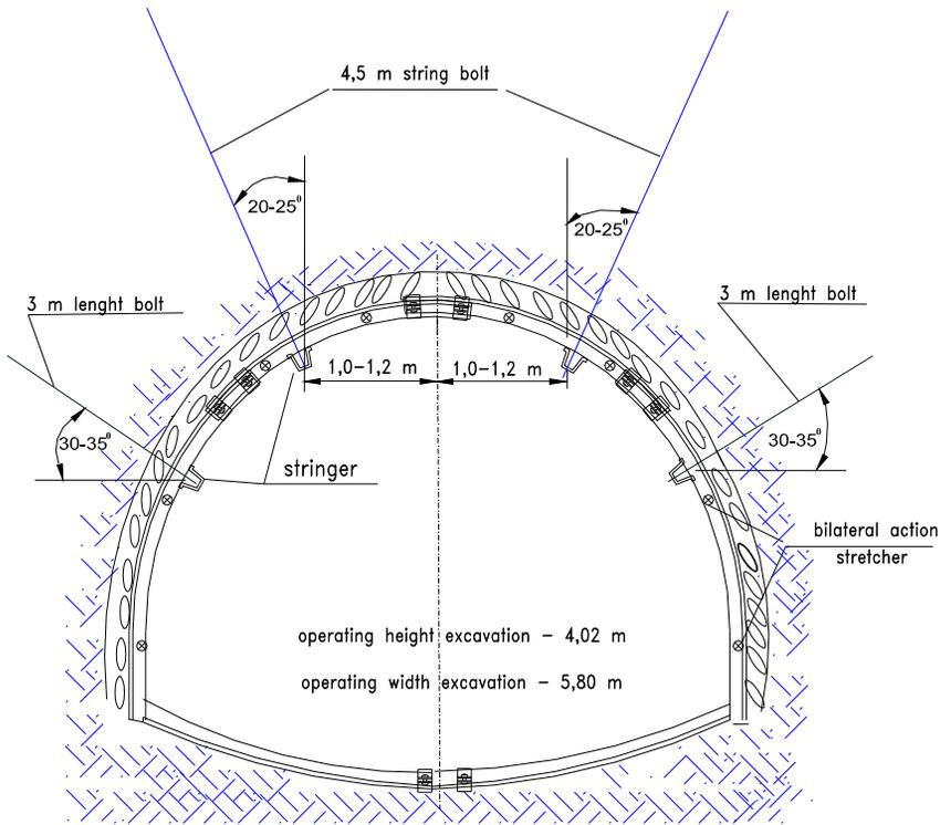
Figure 3. Scheme of cross heading's full support.
