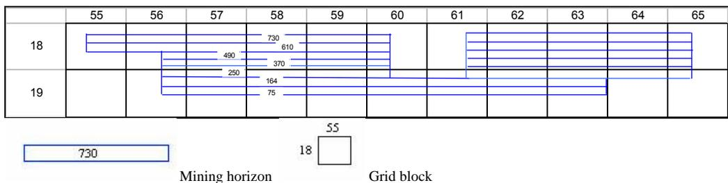
Figure 3. The mine works schedule on the mine named after Rumiantsev over the seam "Yuliev's'ky" according to gridding.
