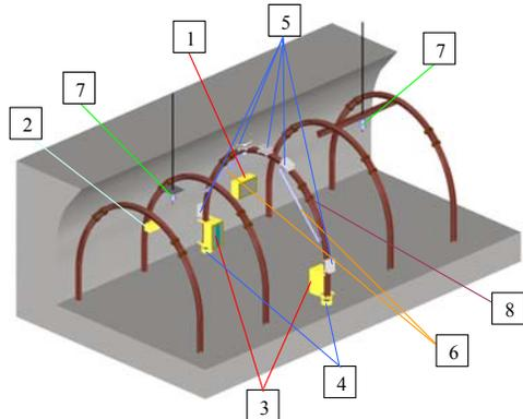
Figure 16. Scheme of monitoring system of roadway support: underground computer (1), module for support deformation measurement by means of the photogrammetric method (2), laser module (3), hydraulic dynamometers (4 and 5), displacement sensors to measure the slide in support friction joints (6), tensometric sensors of bolt load (7), tensometric sensors to measure the force acting at the support shackles' bolts (8). – (Prusek 2008b).
