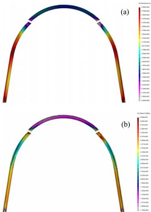
Figure 3. Stress and strain state of the frame support with simulators of the yield locks: (a) distribution diagram of calculation stresses  $\sigma$ ; (b) distribution diagram of horizontal stresses  $\sigma_x$ .
