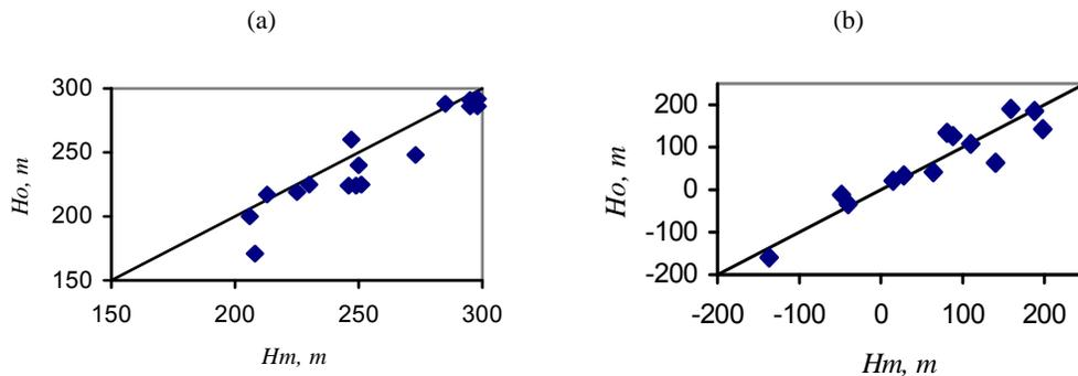
Figure 6. Comparison of modeled ( $H_m$ ) and observed ( $H_o$ ) ground water heads: (a) second layer, (b) fourth layer.
