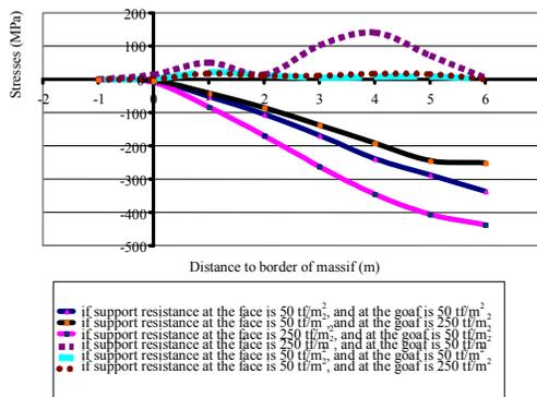
Figure 5. Lines of behaviour of equivalent stresses and roof stone lowering with 0.7 m thickness.
