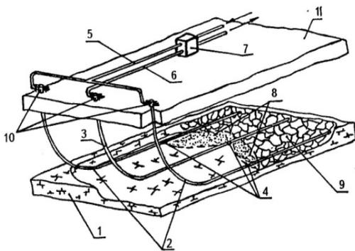
Figure 1. Technological scheme of underground coal gasification from a surface: 1 – coal seam; 2 – injection wells; 3 – production well; 4 – movable ignited devices; 5 – air pipeline; 6 – gas pipeline; 7 – heat – utilization; 8 – combustion face; 9 – goaf; 10 – adjustage of the directed boreholes; 11 – surface.
