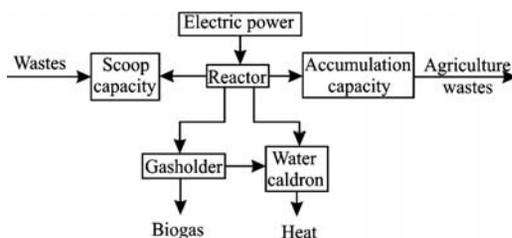
Figure 5. Scheme of setting for the biogas production.
