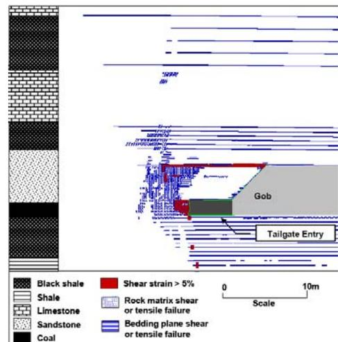
Figure 9. Numerical modeling of the rock mass deformation around the tailgate by means of FLAC program (Esterhuizen, Barczak 2006).
