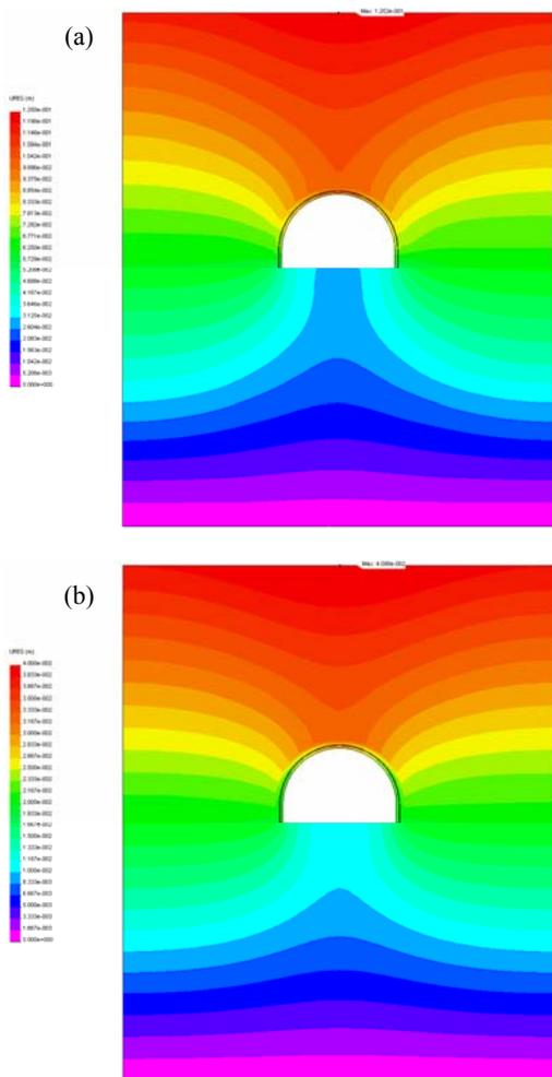
Figure 3. Distribution diagrams of displacements in system “stratified massif-support of working” at increased strength and decreased of deformation characteristics of all adjacent rock layers: (a)  $H = 200$  m; (b)  $H = 600$  m.
