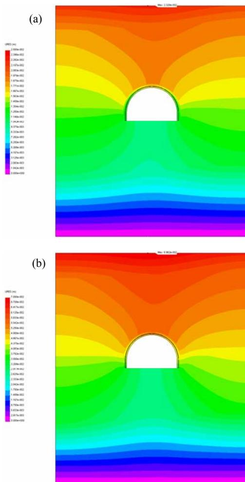
Figure 4. Distribution diagrams of displacements in system “stratified massif-support of working” at increased strength and deformation characteristics of all adjacent rock: (a)  $H = 200$  m; (b)  $H = 600$  m.
