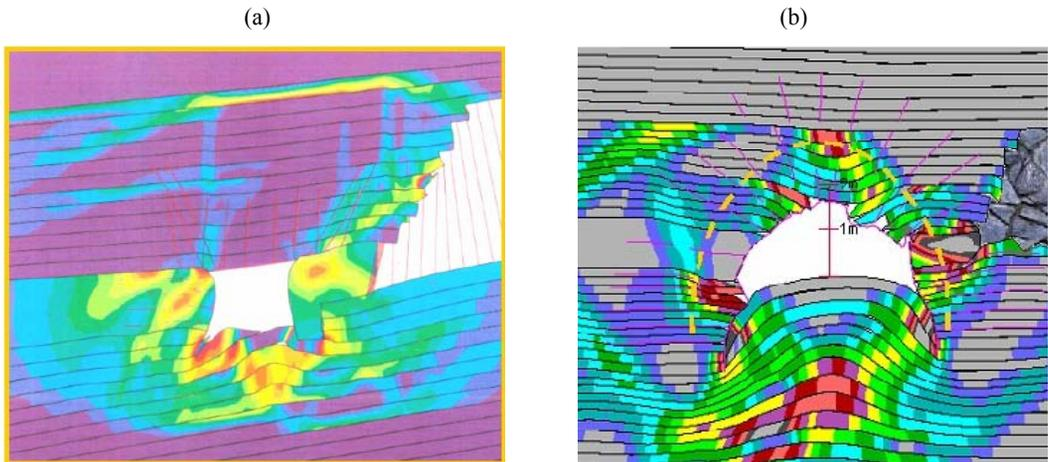
Figure 12. Numerical modeling of gateroad deformation; (a) rectangular bolted gateroad (Langhanki 2001); (b) arch-shaped bolted gateroad (Ruppel & Scior 2008).
