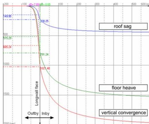
Figure 14. Results of computations of the course of gateroad convergence outby and inby the face based on empirical method worked out at GIG (Prusek 2007).
