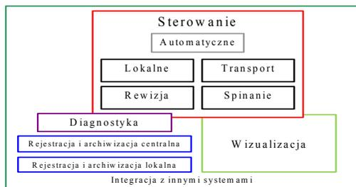
Figure 2.3 (b). Tasks to be carried out by the control system for the plough-based set of extraction machinery.
