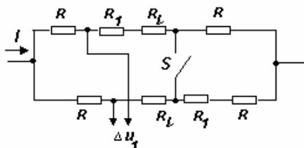
Figure 4. Equivalent circuit for sensitivity assessment.
