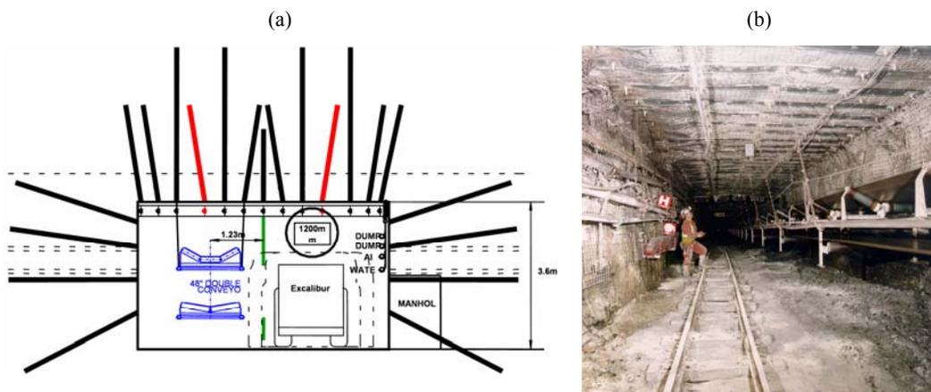
Figure 4. Rock bolted gateroad in one of the UK mines; (a) detailed scheme of rock bolting, (b) view of rectangular rock bolted gateroad.
