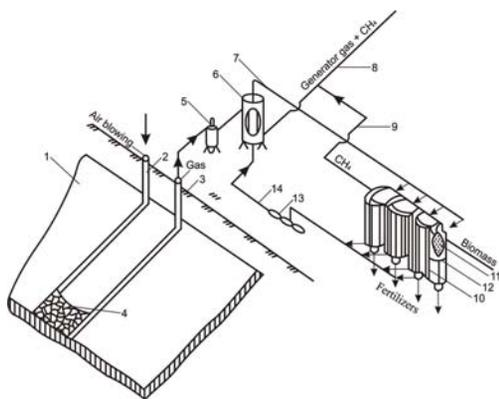
Figure 6. Technological scheme of biogas production with heating of reactors in cold season of year.
