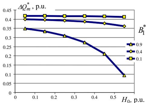
Figure 5. Q-H curves for various stiffness.
