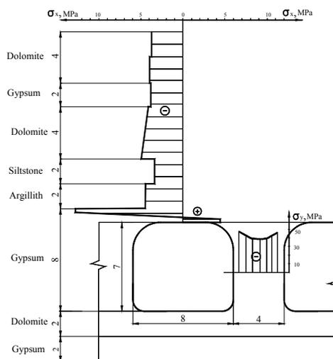
Figure 3. Design diagram and stress eures in roof and pillar rooms.
