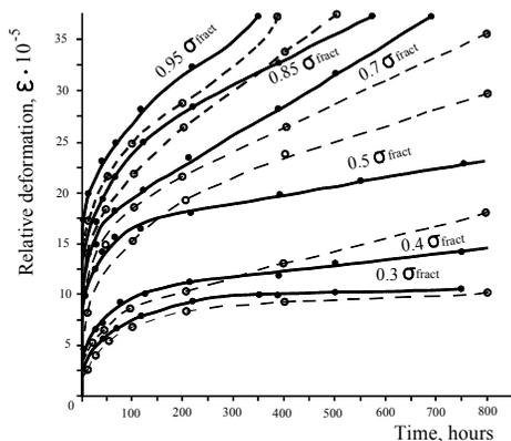
Figure 1. Curves of Gypsum Creep
