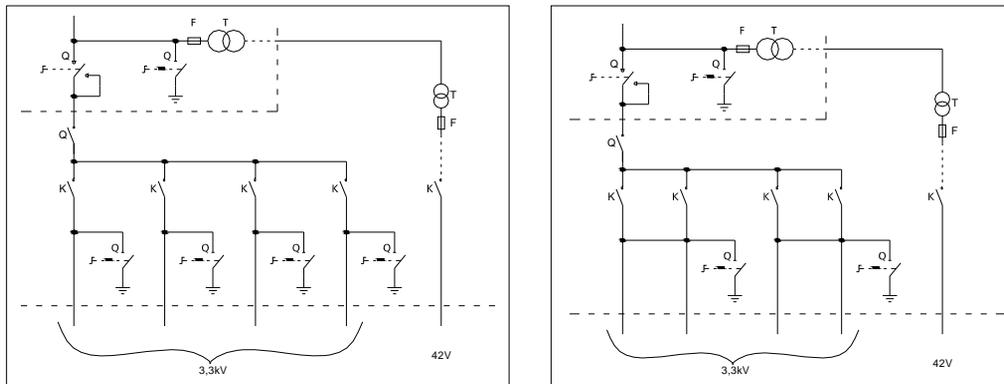
Figure 2.2 (a). The schematic diagram of the four-outlet contactor switch of the type EH-W/3,3/1/01.xx and the schematic diagram of the contractor switch type EH-d03-W/3.3/1/02.xx intended for reversible supply of main motors intended to drive the coal plough.
