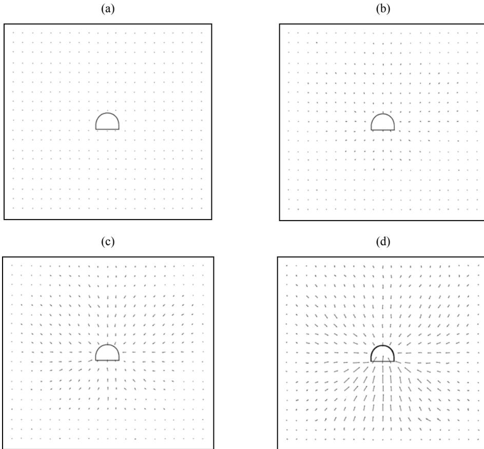
Figure 3. Vectors of angular points displacement on measured grid for homogeneous model at loadings: (a) 0.00 kN, (b) 2.61 kN, (c) 4.56 kN, (d) 7.04 kN.
