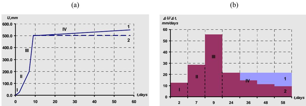
Figure 1. Displacements (a) and speeds of displacements (b) of contour with in meters of “Belozerskaya” of “Dobropol’eugol” (1 – undamping process and 2 – damping process).
