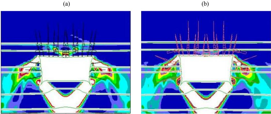
Figure 11. Numerical modeling of gateroad deformation at Daw Mill Colliery; (a) conventional scheme of bolting; (b) scheme of bolting using side wall rock bolts with increased length and diameter (Bowler, Robinson & Altounyan 2009).
