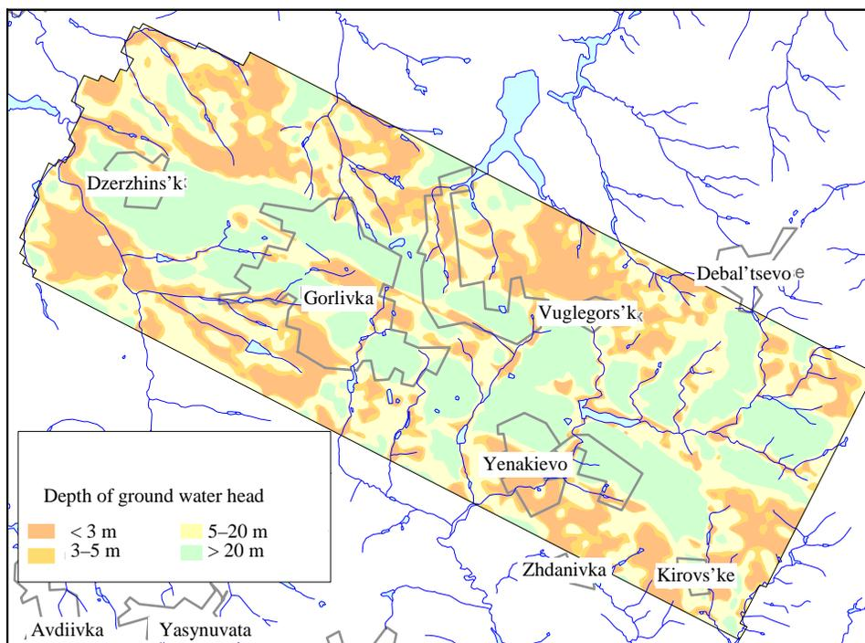
Figure 8. Predicted ground water depth in Central Donbas after mine closure by 2030.
