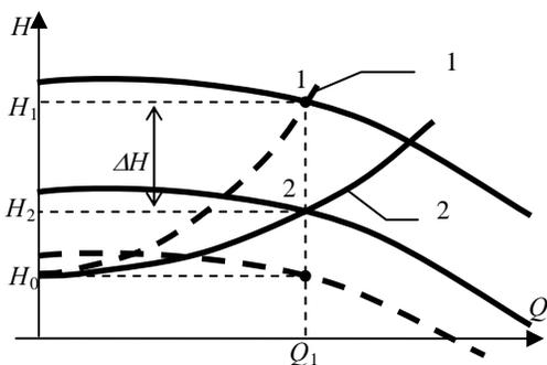
Figure 6. Q-H curves for regulation under various supply.
