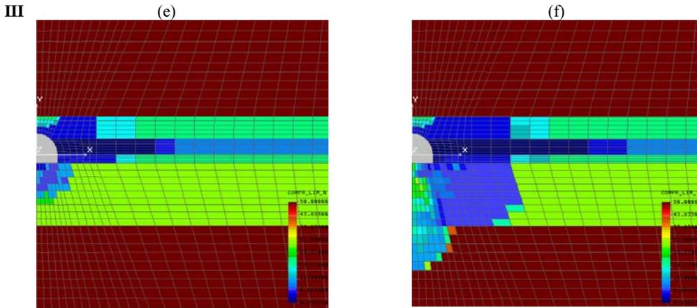
Figure 6. Configuration APD: (a), (c), (e) up to the floor heaving; (b), (d), (f) after the floor heaving, I – homogeneous rock mass including a coal seam; II – rock mass including a coal seam and seam of sandstone in roof (distance between coal seam and sandstone is  $h_{sandst} = 10.0$  m); III – rock mass including a coal seam and seam of sandstone is floor (distance between coal seam and sandstone is  $a_{sandst} = 7.0$  m).
