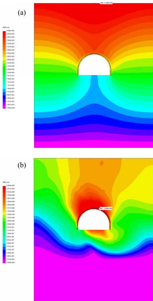
Figure 1. Distribution diagram of displacements in system “stratified massif-support of working” at decreased strength and deformation characteristics of all adjacent rock layers: (a)  $H = 200$  m; (b)  $H = 600$  m.
