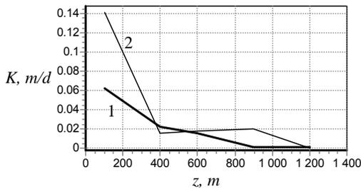
Figure 2. Change of weighted averaged conductivity  $K$  in depth  $z$ : 1 – modeling, 2 – aquifer testing.
