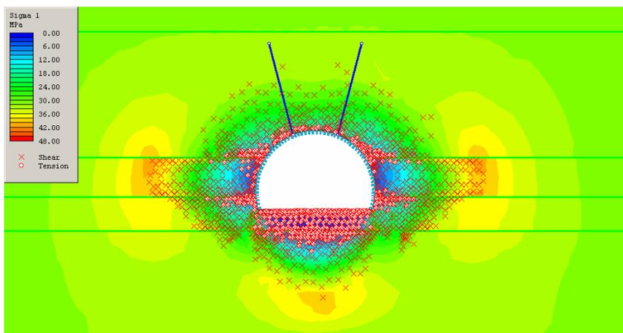
Figure 2. Volume of plastic zone around Cw-1 heading.
