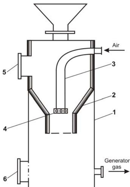
Figure 3. Gasgenerator on the generator gas production: 1 – metallic corps; 2 – cone; 3 – pipe; 4 – snuffed the air serve in the burning zone; 5, 6 – air-tight doors.
