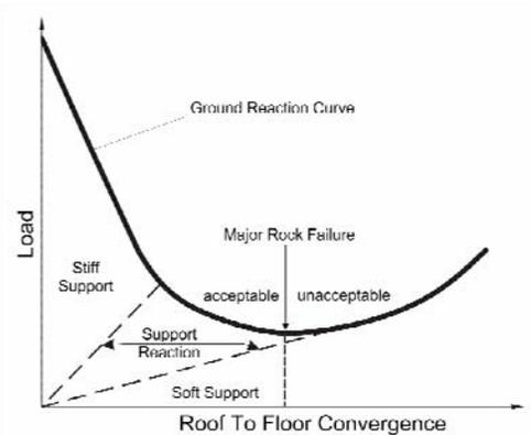
Figure 8. Concept of selecting working support based on the GRC (Mucho et al., 1999).
