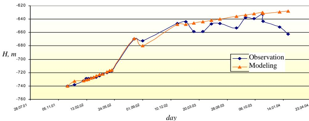
Figure 7. Rise of ground water head  $H$  in coal rocks during flooding of the mine "Chervony Profintern".
