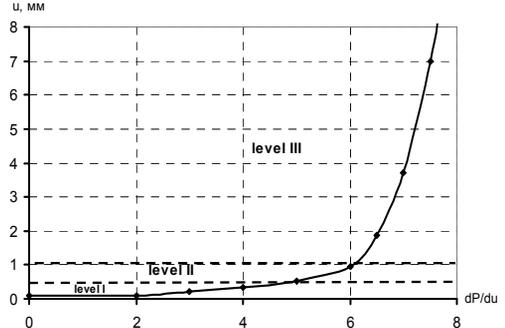
Figure 2. Dependence of floor heaving on the intensity of an exterior loading.
