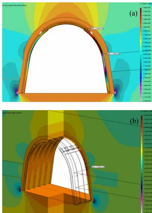
Figure 1. Stress and strain state of the system “rock massif-support” with full reflection of the yield lock’s design: (a) distribution diagram of vertical stresses  $\sigma_y$ ; (b) distribution diagram of axial stresses  $\sigma_z$ .
