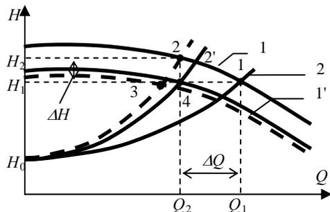
Figure 2. Regulation under constant pressure.
