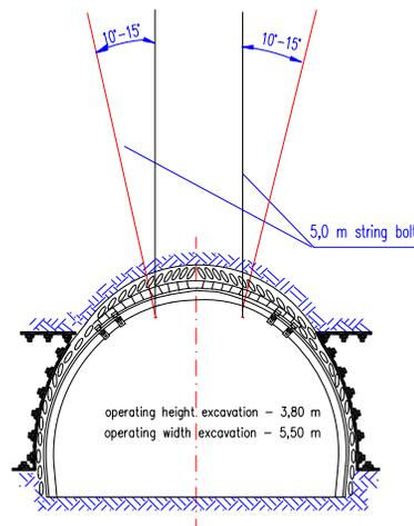
Figure 1. Support scheme for Cw-1 heading.
