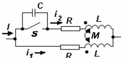
Figure 2. Equivalent circuit for assessment of energy liberated in the discharge.
