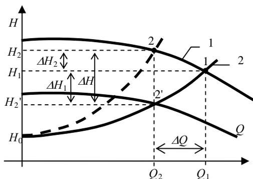
Figure 4. Regulation under variable pressure and supply.
