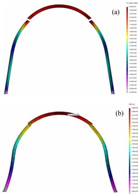
Figure 4. Stress and strain state of the frame support with simulators of the yield locks: (a) distribution diagram of vertical stresses  $\sigma_y$ ; (b) distribution diagram of full displacements  $U$ .
