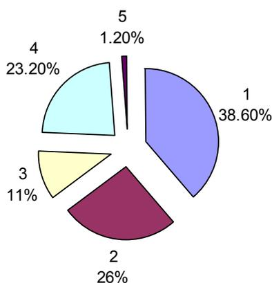
Figure 5. Calculated balance components of water inflow to mine in 1990: 1 – recharge, 2 – storage, 3 – shortening of ground water runoff, 4 – surface water inflow, 5 – shortening of infiltration.
