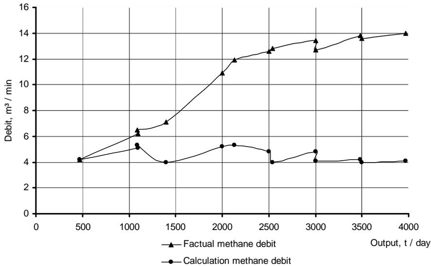
Figure 2. Dependence of methane distribution in workings on coal production rate.
