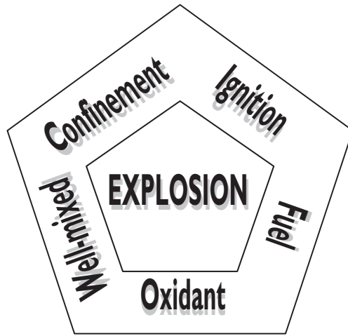
Figure 6.6 Ingredients Fuel, Oxidant and Ignition-source, when well mixed and having proper confinement result a successful explosion or blasting operation.
