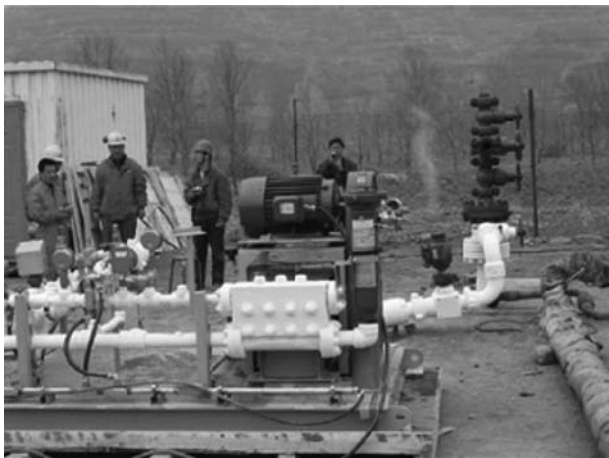
Figure 10. Injection of liquid CO 2 at the project site of micro-pilot test at Qinshui (Gunter et al., 2005).
