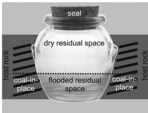
Figure 2. The different elements of the jar pot model, with the partially flooded residual space corresponding to the jar. Coal-in-place is adjacent to the jar. The natural and man-made sealing of the reservoir is represented by the seal of the jar, which can move in respect to the reservoir pressure to simulate the effects of absidence.
