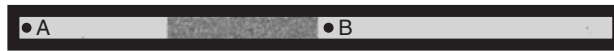
Figure 12.22 Numerical model of the sample and transmitter bars ( 400 \times 15 elements with 5 mm length scale for the element).
