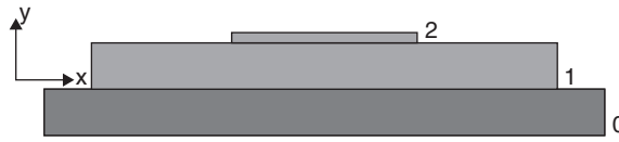
Figure 16.2 The modeled DDA block system constraining the motion of Block 2 to horizontal sliding only. Block 0 is the foundation block, Block 1 receives the dynamic input motion (horizontal – cyclic), and Block 2 responds (after Kamai and Hatzor, 2008).
