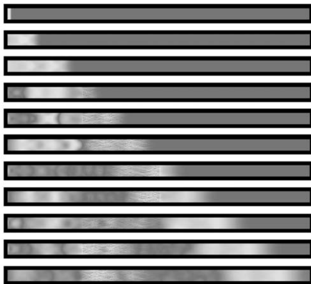
Figure 12.24 Numerically obtained stress wave propagation along the bars and the sample with m = 2 .
