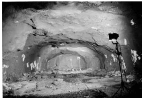
Chamber after detonation (Test #4b)
