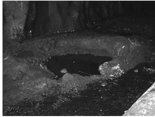
Chamber with craters after detonation (Test #3)
