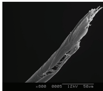
Fig. 9. External cracks after fatigue test (Cotton I)
