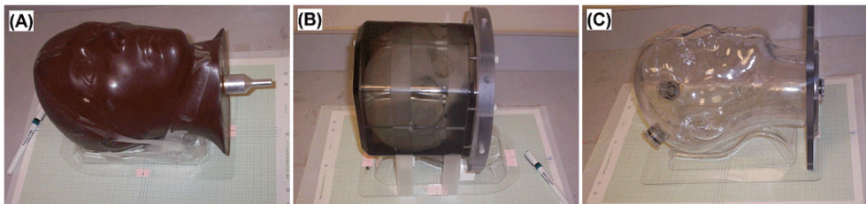
Fig. 8. Three anthropomorphic head phantoms for CT (A), MRI (B), and PET/CT (C) imaging.
