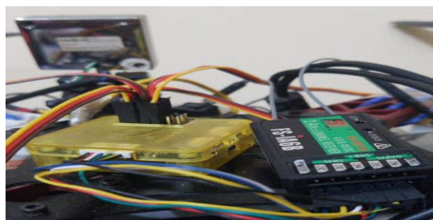
Fig 5.3: Flight controller (CC3D) and receiver wiring.
