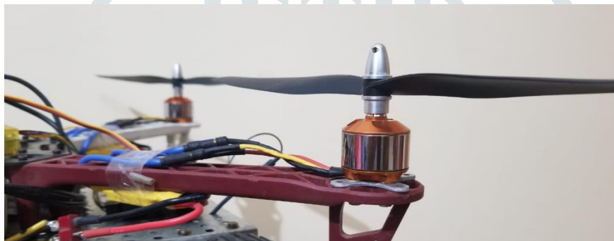
Fig 5.2: Motor and ESC mount.
