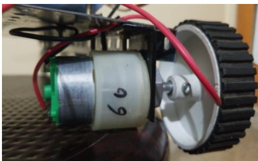
Fig 5.6: Motor used for driving the wheel
