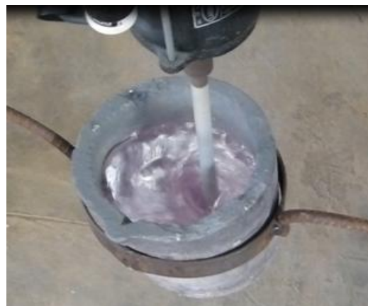
Fig. 1. The molten metal was stirred to create a vortex
