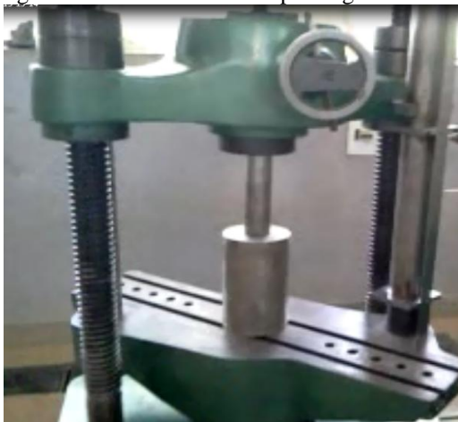
Fig. 3. The molten metal was squeezed using plunger
