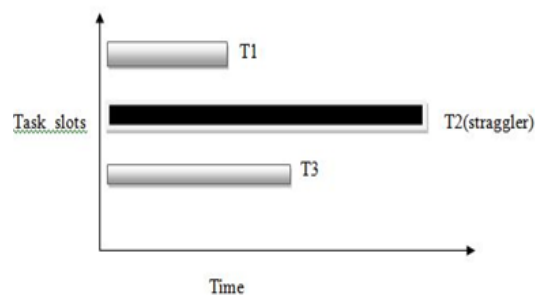
Fig.4. Data Skew caused due to straggler (without skewtune)
