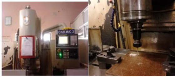
Fig 1. CNC drilling machine drilling hole on JFRP PU-foam composite
