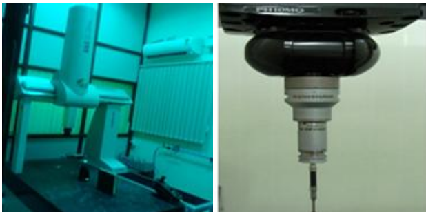
Fig 3. Coordinated Measuring Machine (CMM) Motorized automated probe
