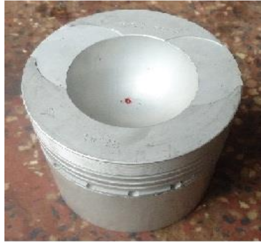
Hemispherical piston bowl geometry (HPBG)
