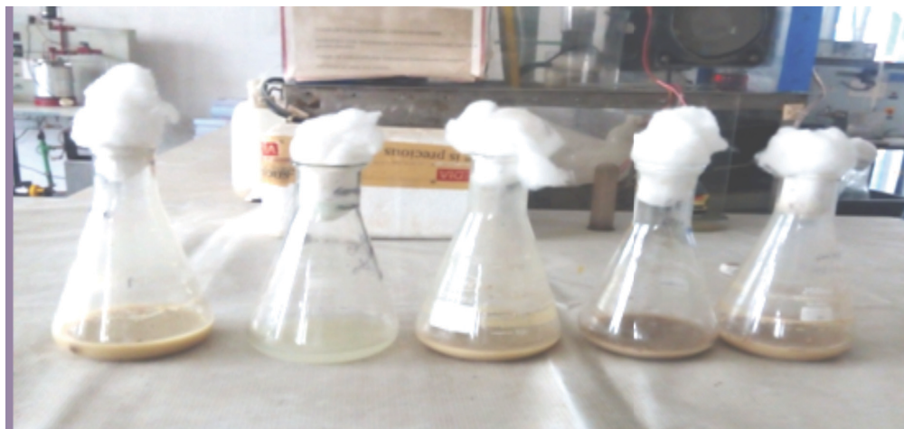
Fig. (2). Biodegraded plastic samples after 35days of incubation.
