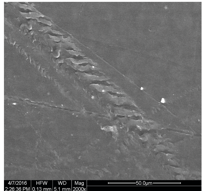
Fig. (8). SEM analysis showing surface degradation of white plastic incubated with unknown fungi.
