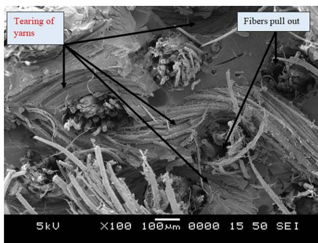
Figure 22. SEM image fractured surface of P1 based composites under impact loading.
