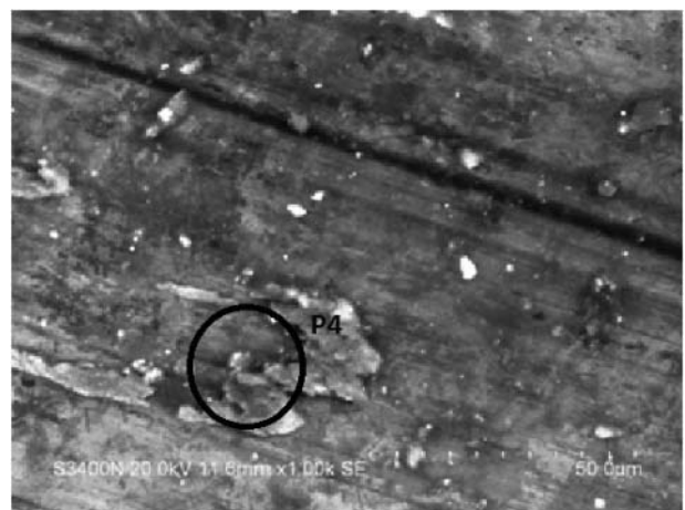
Fig. 6d—SEM showing wear track morphology of 3% SiC and 3% graphite composites at 1.047 m/s and load of 80 N.
