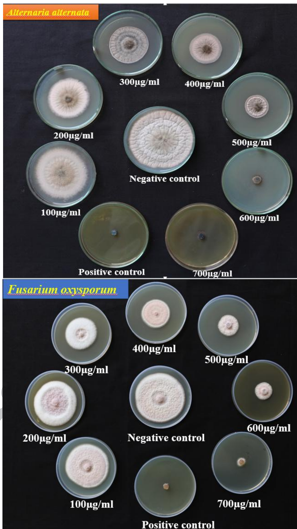
Fig.24. Antifungal activity of ZnO:Nd 3+ Nps against Plant pathogenic fungi Alternaria alternata and Fusarium oxysporum .
