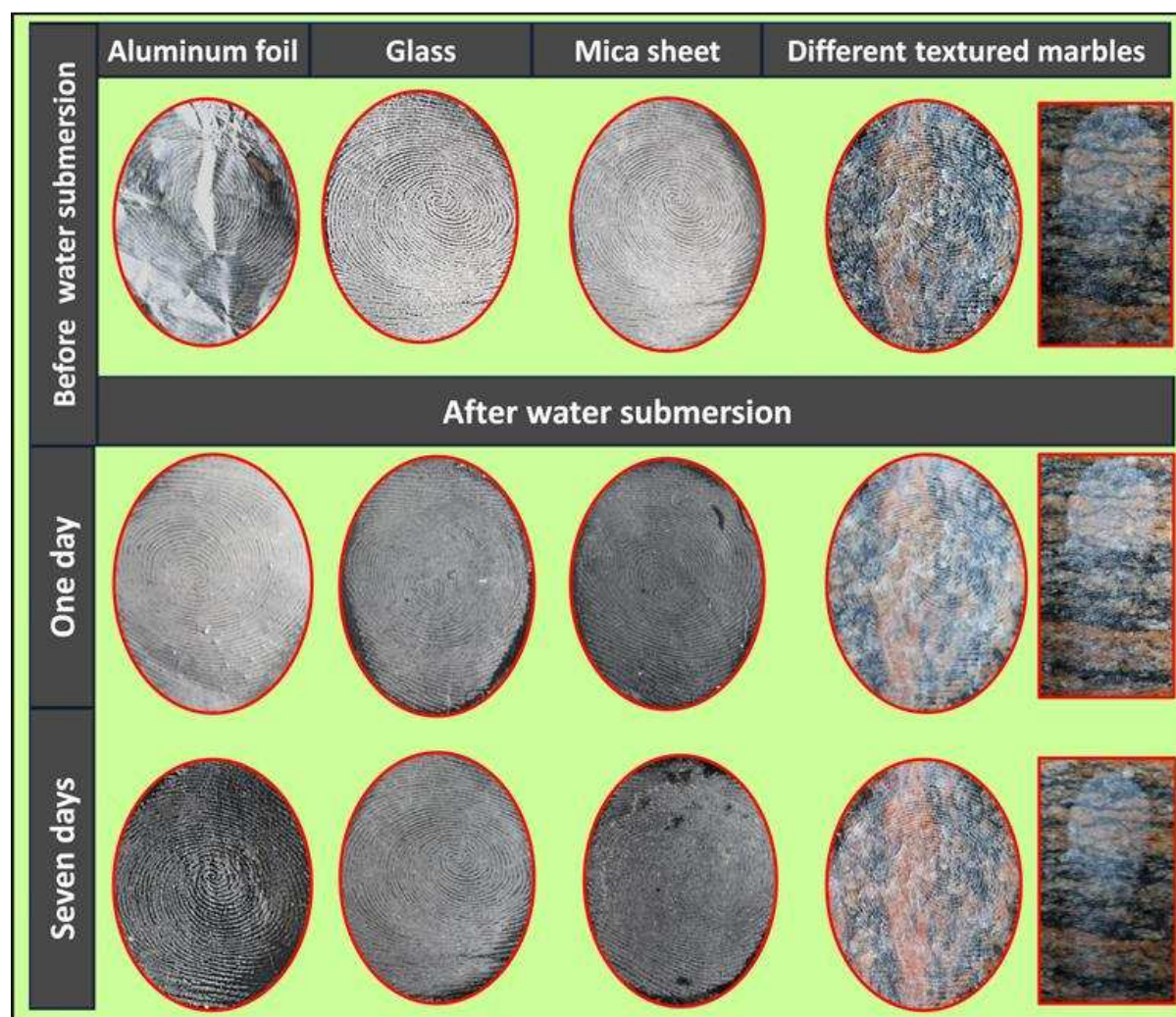
Fig.11 Developed FPs using optimized C-dot@TiO 2 (III coat) NSs on various substrate surfaces: aluminum foil, glass, mica sheet and textured marbles before and after submersion in fresh water for one and seven days.
