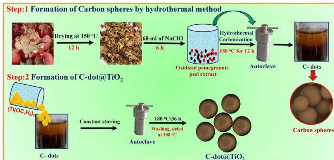
Fig.1. Schematic illustration for the formation of C-dots from the hydrothermal treatment of pomegranate waste peels and C-dot@TiO 2 nanostructures.
