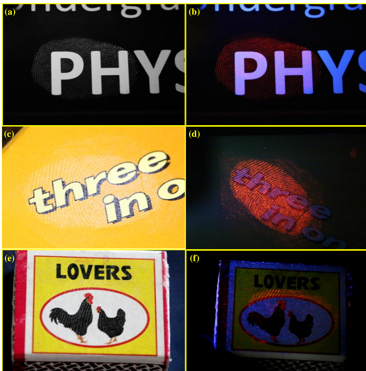
Fig.18(a-f) LFPs visualized by \text{CeO}_2:\text{Eu}^{3+} (3 mol %) NP on various surfaces of paper substrates with different background colors.
