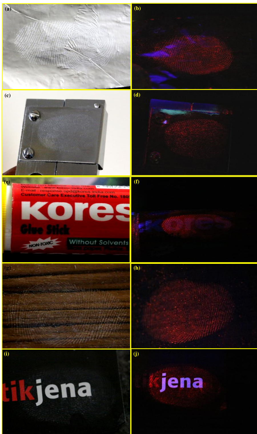
Fig.17. LFPs visualized by \text{CeO}_2:\text{Eu}^{3+} (3 mol %) NP on (a & b) aluminum foil (c & d) stainless steel, (e & f) plastic sheet, (g & h) wooden floor sheet and (i & j) compact disk cover under normal visible and UV 254 nm light respectively.
